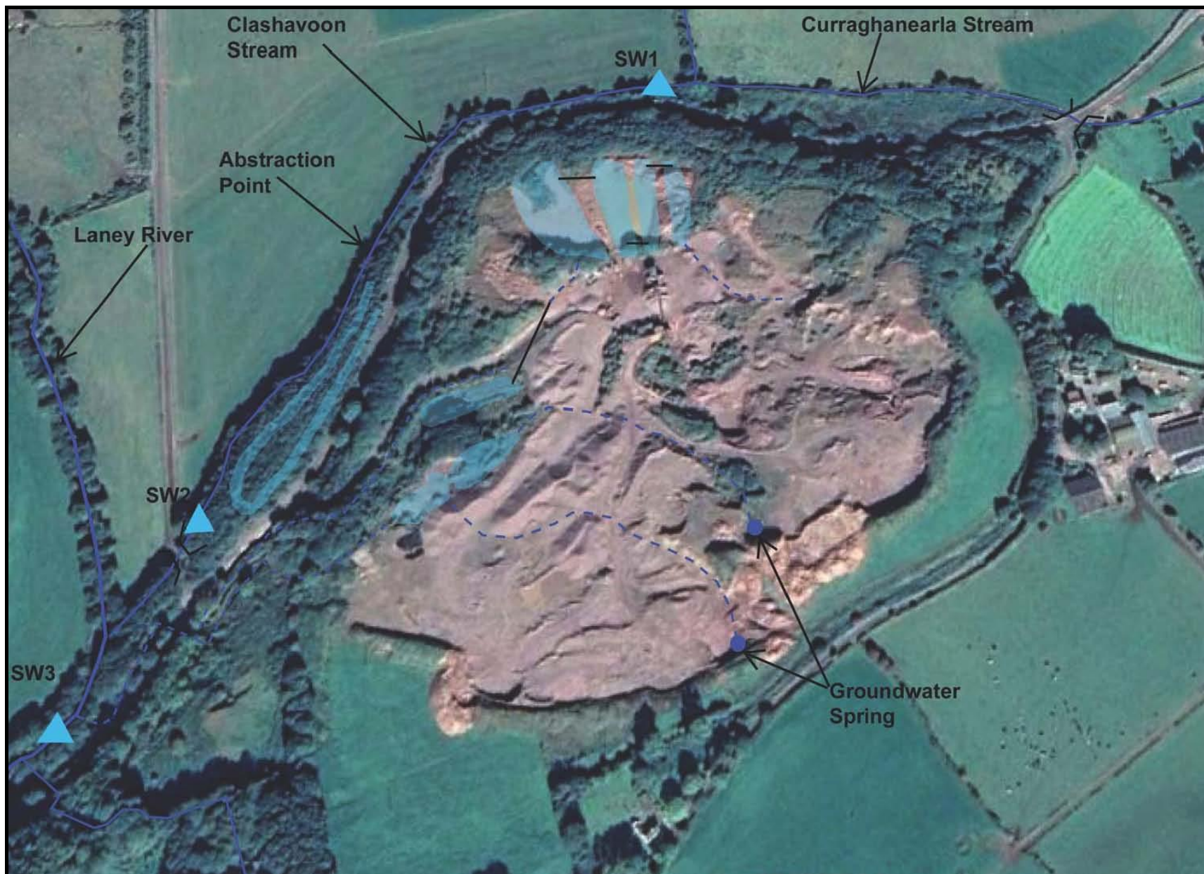
Figure 7-2: Local Surface Water Drainage
